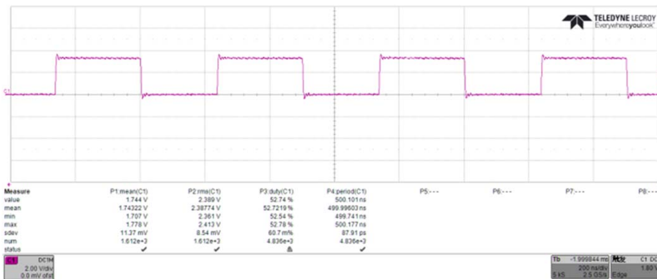
Fig. 4 Output duty ratio when input data=4295
