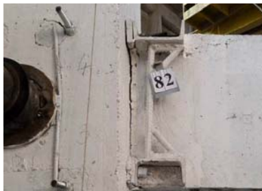
Fig. 10 Rotation of the beam in modified hybrid joint at a drift ratio of 0.027, respectively a top displacement of 81mm
