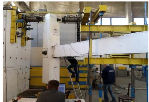
Fig. 12 Self-balancing property of spatial model
