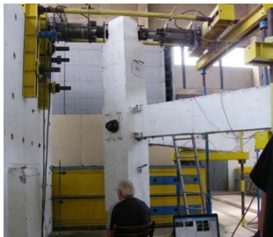
Fig. 11 Deformed configuration under loading
