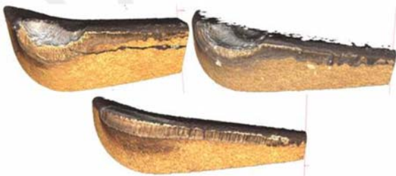
Fig. 4 High resolution 3D scans of tools after 15 minutes' turning
