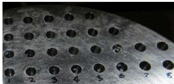
Fig. 5 Array of blind drilled holes in test piece surface
