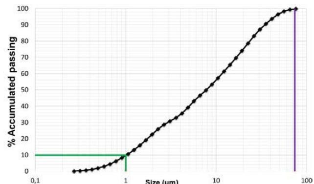
Fig. 3 Particle size analysis average limestone fines
