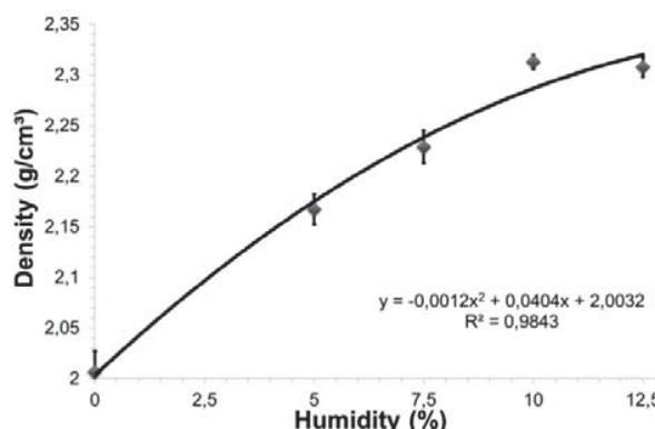
Fig. 6 Variation of the density of briquettes relative humidity
