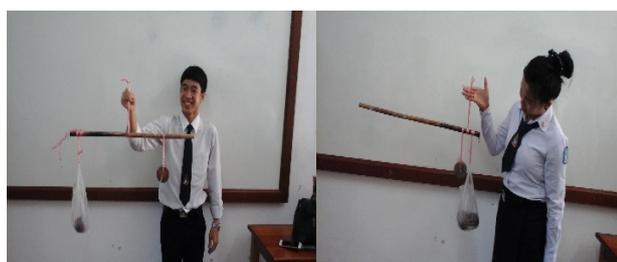
Fig. 3 Mass measurement by balance of two kinds
