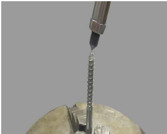
Fig. 4 Spike used for calibration of the rotational table
