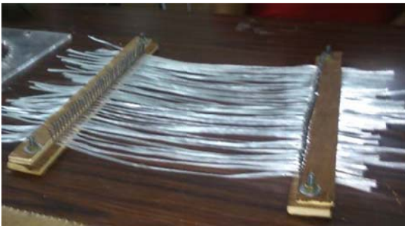
Fig. 2 Fiber alignment in clamps
