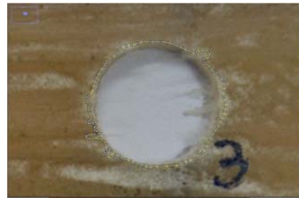
Fig. 4 Delaminated hole for hole 3
