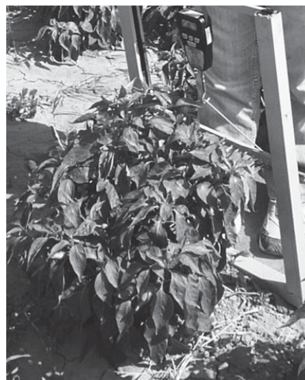
Fig. 3 Force measurements with experimental harvest mechanism
