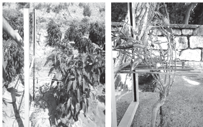
Fig. 2 Manually actuated experimental harvest mechanism
