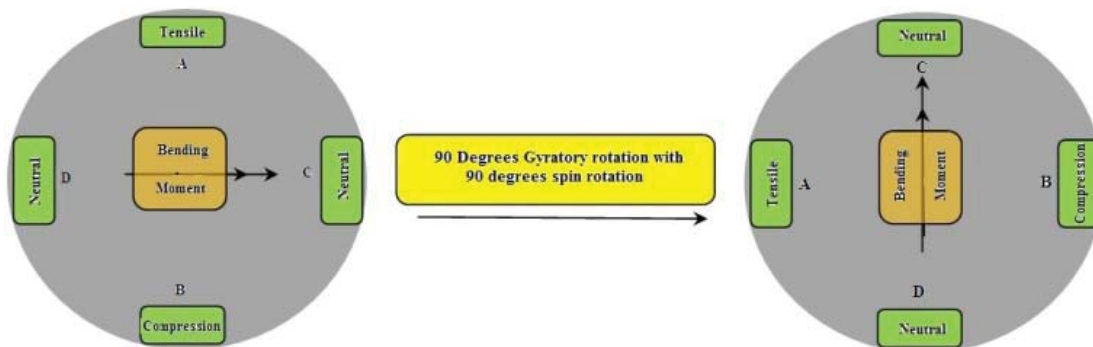
Fig. 5 Stress condition when Gyratory movement and rotational spin are synchronized
