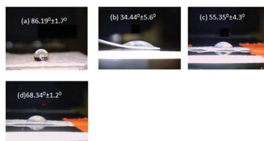
Fig. 4 WCAs of MTAMs (a) untreated, (b) P.D. acetic acid (c) S-Graft AAc (5%), and (d) chitosan Immobilized
