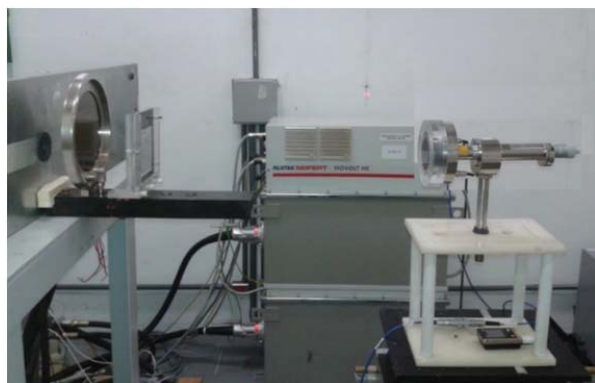
Fig. 1 X-ray set-up for measurements with the 23392 PTW extrapolation chamber
