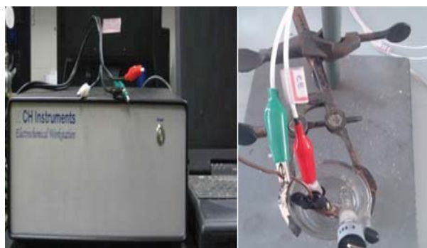
Fig. 3 CH instrument used for measuring the rate of corrosion
