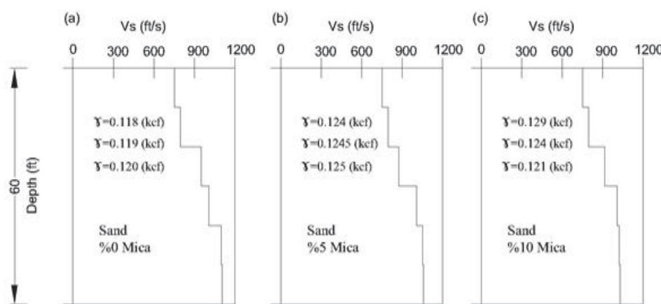
Fig. 1 Shear wave velocity, unit weight, and mica content variations for the soil profile
