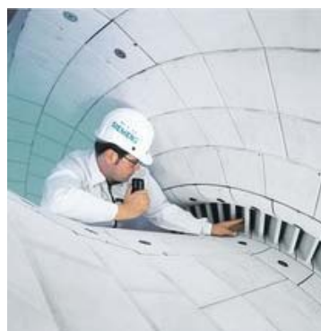
Fig. 1 Inspection of heat tiles in the combustion chamber from Siemens
