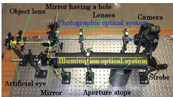
Fig. 2 Experimental device
