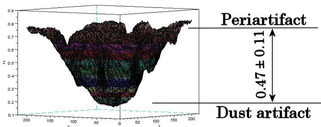
Fig. 11 V value for dust artifacts visualized in the artificial eye with a rose-colored fundus
