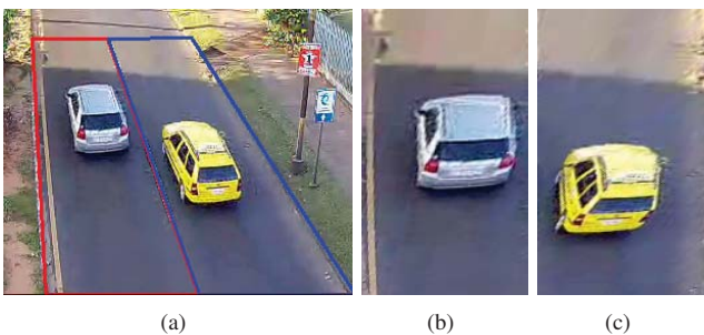
Fig. 5 Results obtained after applying the perspective correction. In (a) the counting regions defined in the step of image acquisition are observed. The perspective correction from both lanes are observed in (b) and (c)
