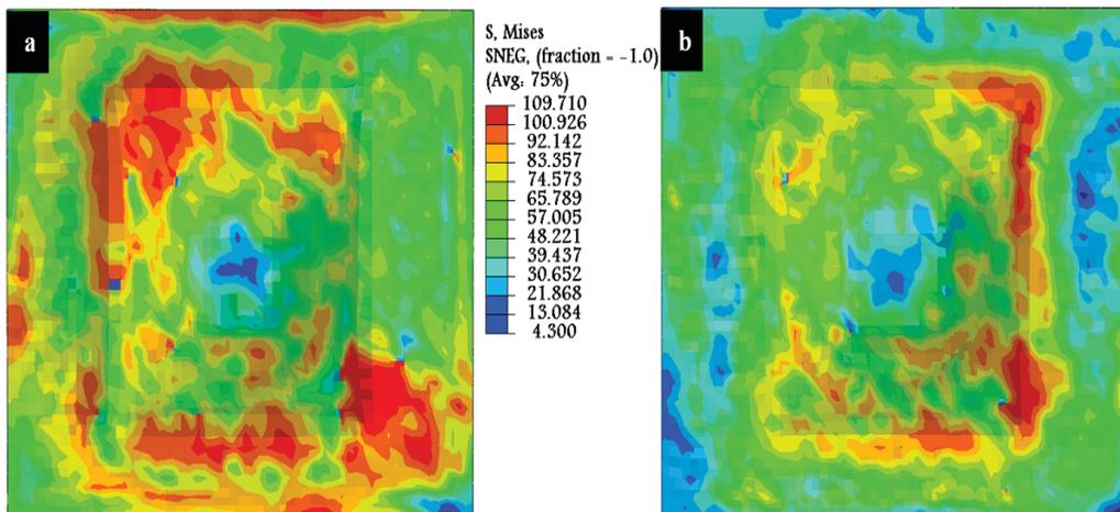
Fig. 9 Stress distribution in the part (a) without an interpolator (b) with an interpolator
