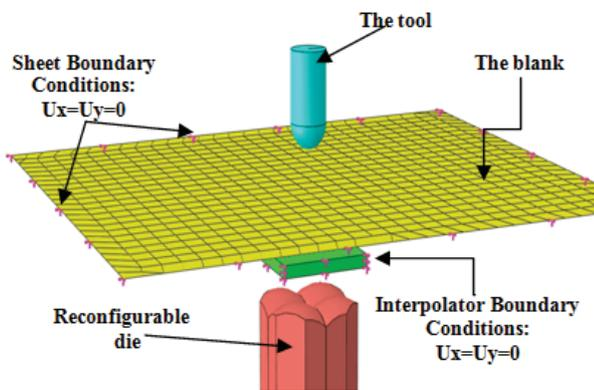
Fig. 5 Numerical model of the MPIF process
