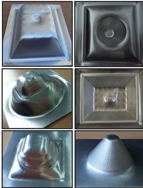
Fig. 3 Parts manufactured using the MPIF process
