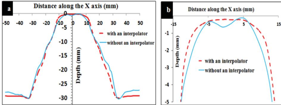
Fig. 8 Influence of the elastomeric interpolator
