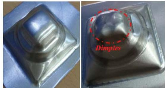
Fig. 7 Influence of the elastomeric interpolator
