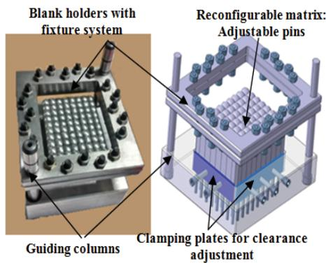
Fig. 2 Experimental set up of the MPIF process
