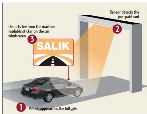
Fig. 1 A toll payment system in Dubai, called SALIK, using RFID technology [1]
