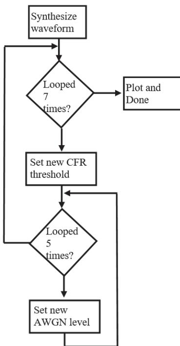
Fig. 1 Flow chart of the simulation algorithm
