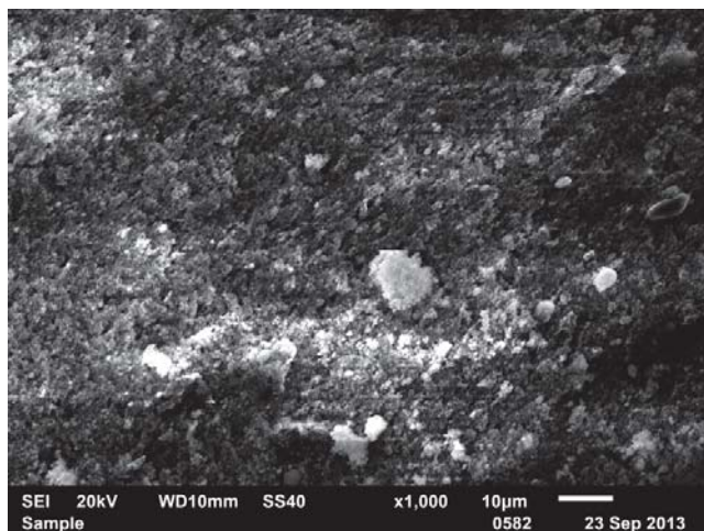
Fig. 2 Electron micrograph of thermal treated catalyst
