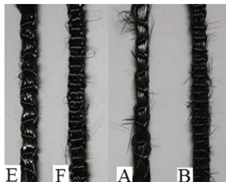
Fig. 5 Non-crimp 3D orthogonal weave samples
