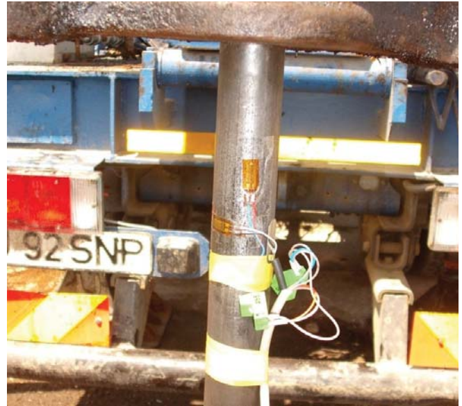
Fig. 6 Accelerometer sensor placed on the oil pumping unit polished rod
