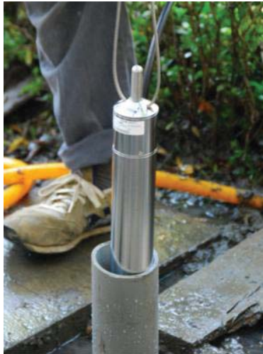
Fig. 3 A seismometer was installed in the downhole with a depth of 40 meters in the third stage.
