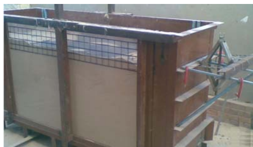
Fig. 3 Sand container and lateral stressing mechanism
