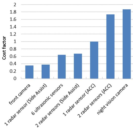
Fig. 4 Repair cost analysis of ADAS sensor types
