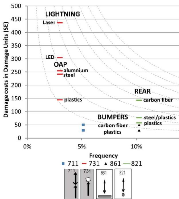
Fig. 3 Material parameter analysis for property damage risk [7], [16]
