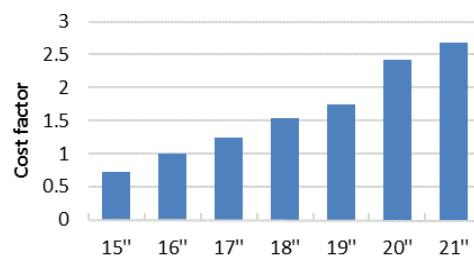
Fig. 8 Repair cost analysis of rim size
