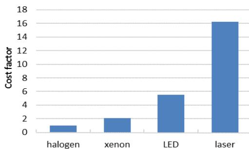
Fig. 7 Repair cost analysis of headlight types
