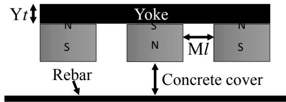
Fig. 8 Proposed structure of the adhesion module
