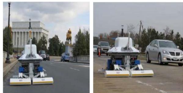
Fig. 3 Operation of GPR bridge deck assessment robot [14]
