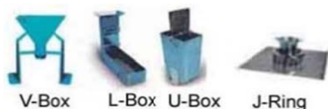
Fig. 4 Fresh concrete testing devices
