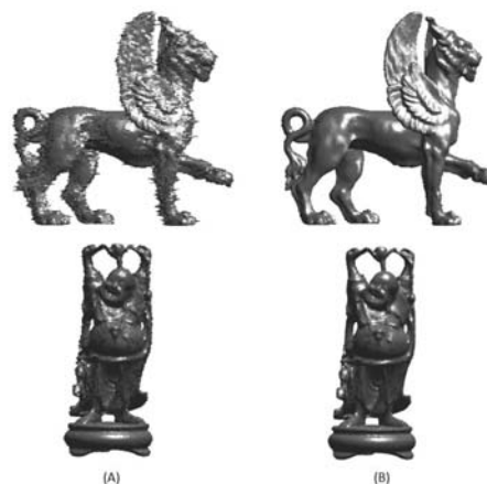
Fig. 5 The Results of 3D reconstruction with the following number of POLYWOG wavelets ((A):300 wavelets, (B):350 wavelets)
