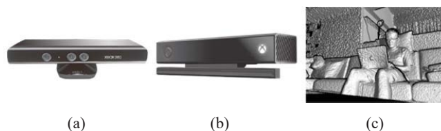
Fig. 1 (a) First generation Kinect-Kinect360, (b) second generation Kinect-Kinect V2, (c) depth information obtained by Kinect V2
