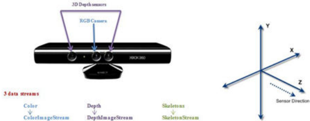
Fig. 2 Kinect Sensor and coordinate system
