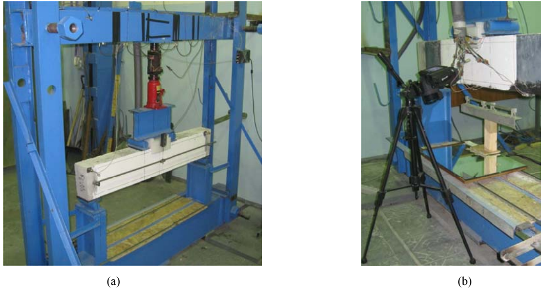
Fig. 2 Test set-up equipment: the test set-up with a loading tool (a) and the infrared shooting scheme (b)
