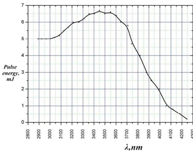
Fig. 2 Tuning curve of KTA-based OPO in the 3–4  $\mu\text{m}$  range
