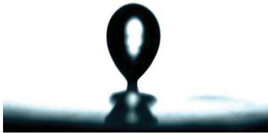
Fig. 5 Bubble just before detachment
