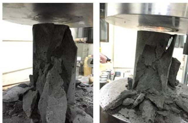
Fig. 5 Fracture aspect of 7 days compressive strength
