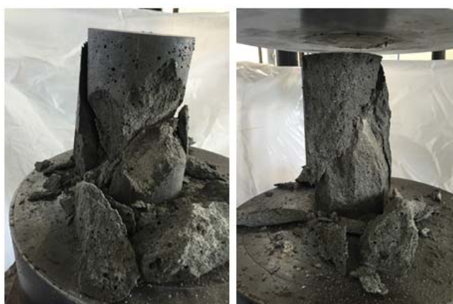
Fig. 6 Fracture aspect of 28 days compressive strength
