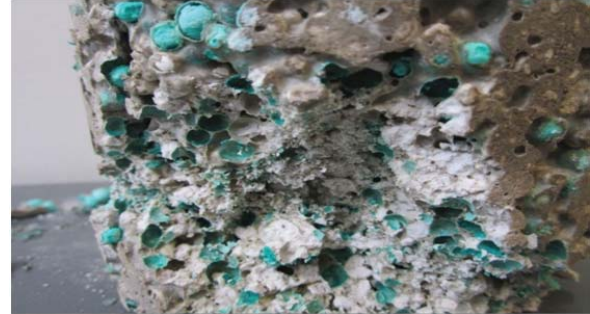
Fig. 2 Effect of alkaline environment on PLA aggregate
