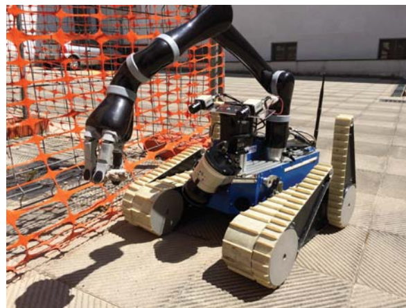
Fig. 1 Actively Articulated Tracked Vehicle Absolem, designed by ©Bluebotics [4] for USAR applications: This platform is equipped with the KINOVA Jarm Arm for pick and place operations
