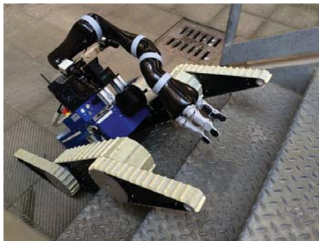
Fig. 2 Actively Articulated Tracked Vehicle Absolem, designed by ©Bluebotics for USAR applications. This platform is equipped with the KINOVA Jarm Arm for pick and place operations
