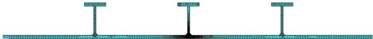
(b) Finite element mesh model for three continuous stiffener
