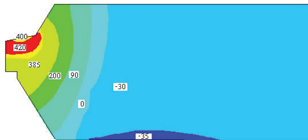
(a) Residual stress contour of critical points
