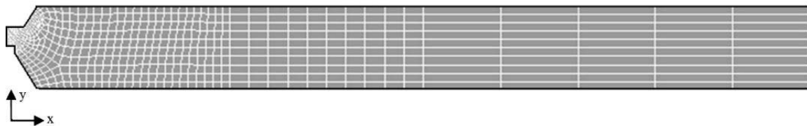
Fig. 4 Plate 2D finite element mesh
