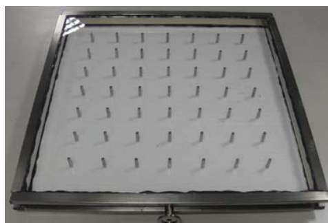
Fig. 9 Fabricated flat vacuum panel
