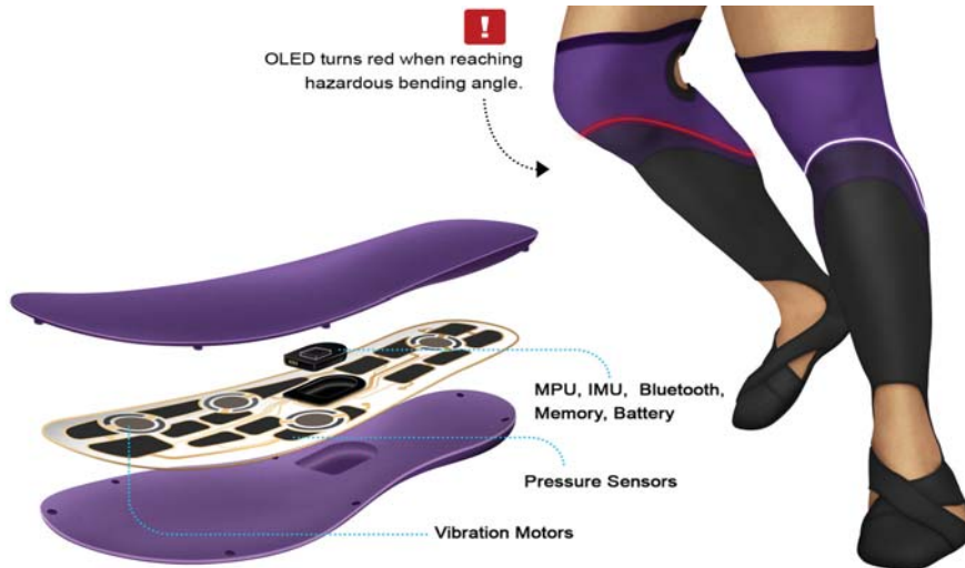
Fig. 4 Hands-free feedback delivers to insoles and kneepad by vibrations and lightening
