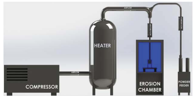
Fig. 2 Schematic representation of the high temperature erosion testing rig
