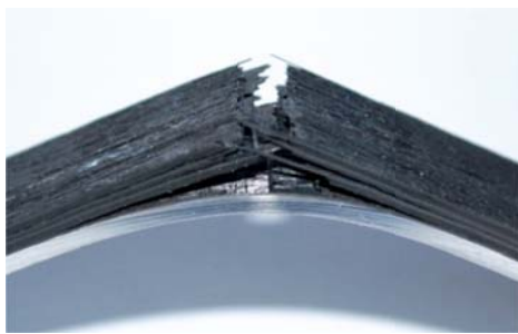
Fig. 4 Failure behaviour of hybrid three-point bending samples (force transmission from the side of the sheet metal)
