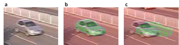
Fig. 6 Impact of both weighting strategy and normalization operation on vehicle matching: (a) Test image, (b) Matching result with the weighting strategy and normalization operation, (c) Matching result without the weighting strategy and normalization operation
