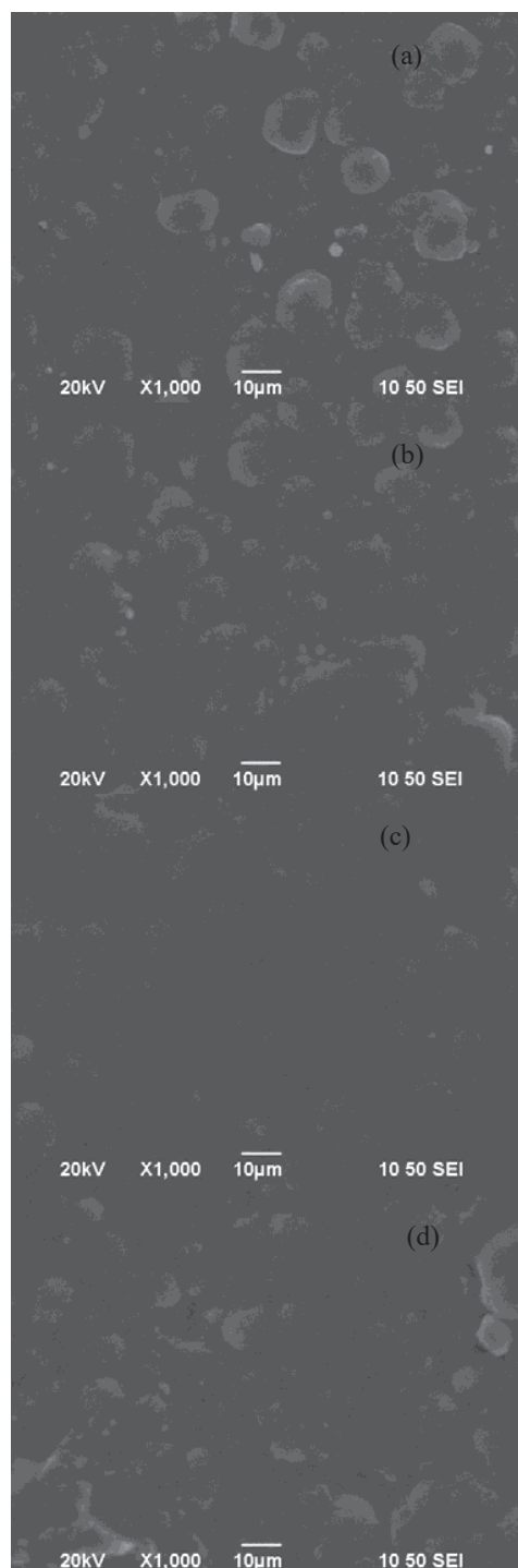
Fig. 4 SEM pictures of polyurethane synthetic leather, after plasma treatment with different amounts of TMS: (a) 0.1ml, (b) 0.15ml, (c) 0.20ml and (d) 0.25ml. (Process parameter: Treatment dwell time = 30 seconds, Flow rate of helium = 7.5 LPM, Jet distance = 10 mm and Discharge power = 50W)
