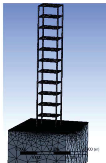
Fig. 1 Fixed base model and model with soil-structure interaction after generating mesh in ANSYS
