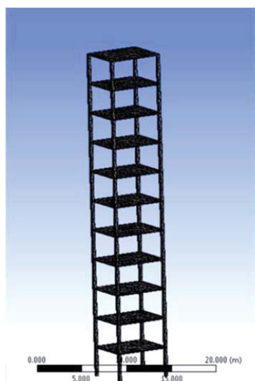
Fig. 1 Fixed base model and model with soil-structure interaction after generating mesh in ANSYS
