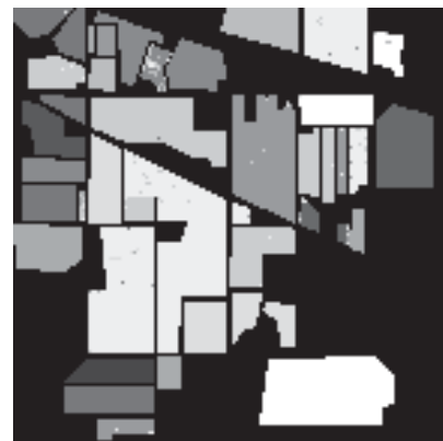
Fig. 6 Segmented image by GMLC with all bands (220 bands)
