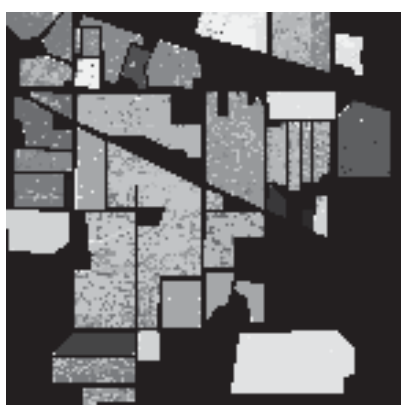
Fig. 8 Segmented image by GMLC with 17 bands selected by FCM with Variance and Kurtosis
