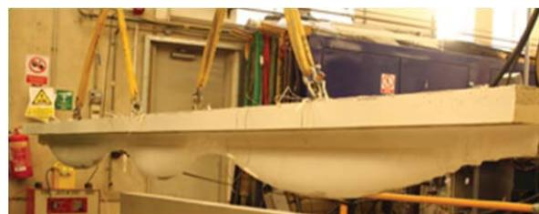
Fig. 1 Fabric-formed concrete
