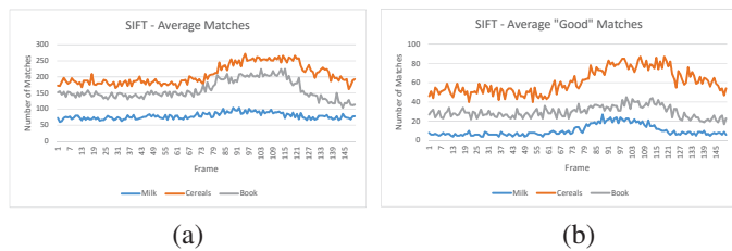
Fig. 13 SIFT descriptors matching: (a) Number of matches; (b) Number of "good matches"
