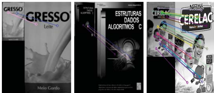
Fig. 14 SURF descriptors matching: Colored lines represent the "good" matches
