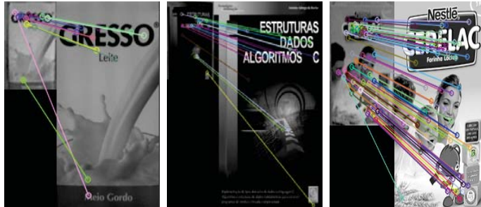
Fig. 12 SIFT descriptors matching: Colored lines represent the "good" matches
