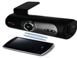
Fig. 4 Setting function values in a blackbox using NFC
