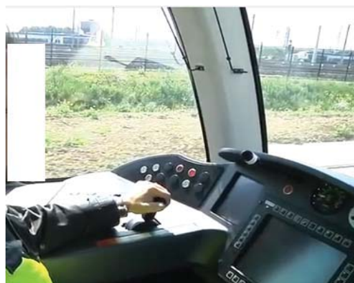
Fig. 2 A physical effort (handlebar) causing fatigue to the conductor's tram [6]
